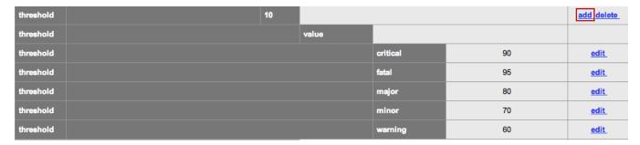
Complete the details in the control "\$ifSpeed <= 5000000 and \$ifSpeed >= 1000000" and click add.
