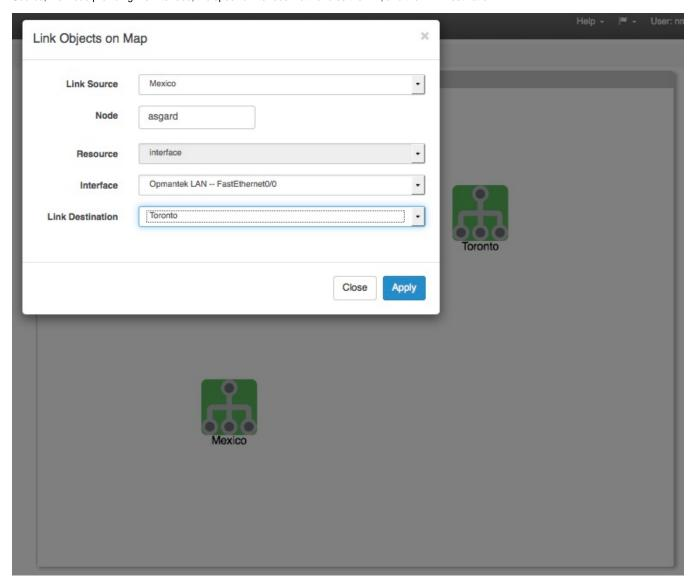
The resulting link will be anchored to the 2 Nodes/Groups and display both the inbound and outbound link speeds as a percentage of the available interface speed. The link is also hinged in the middle, allowing some modicum of adjustment for background artwork and readability.
