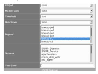
Notice that via the GUI edit node context you can select multiple nodes for the depend value. This may be advantageous if the site has redundant edge routers.
