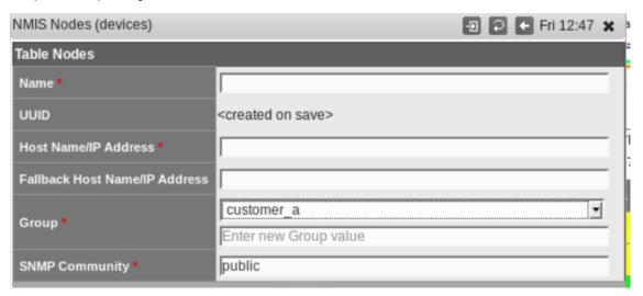
Notice the group section is comprised of two different input fields. The first one is a drop box containing all the currently configured groups. If the Node's group is not in this drop down box, we can enter a new group value in the text box below it.
